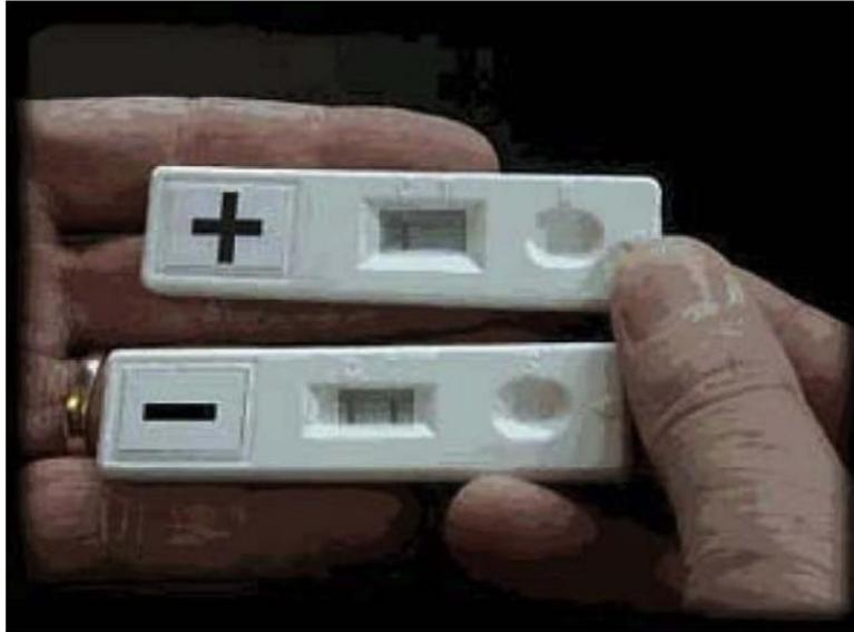
*Figure 9: Jellett MIST test strip for rapid and simple PSP toxin detection (Source: [20])*
