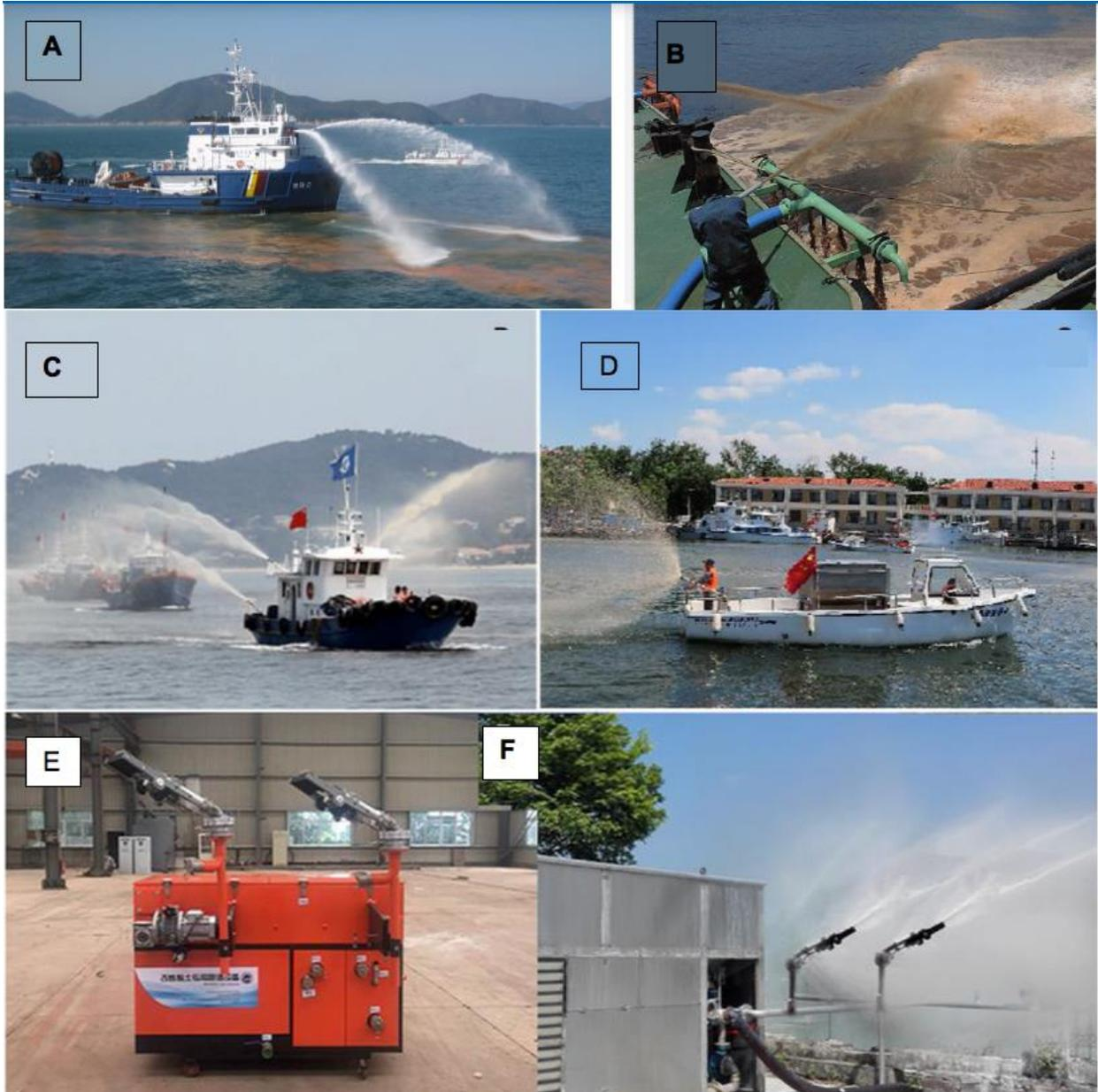
Figure 6: Ships and machines for dispersing clay. A. South Korean vessel spraying clay; B. South Korean vessel with large manifold at the rear of the ship for clay dispersal; C. Chinese vessels spraying clay; D. Small boat designed specifically for clay dispersal (Source: [23])
